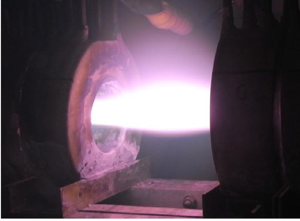
Fig. 4. A photograph of the plasma flow in the mirror magnetic field.
