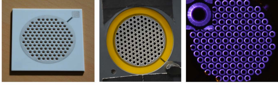
Fig. 2. Photographs of the plasma discharge array prototype (left), mounted at the jet exhaust (center) and powered by an AC voltage with amplitude of 14 \text{ kV}_{p-p} at 2000 \text{ Hz} (right).
