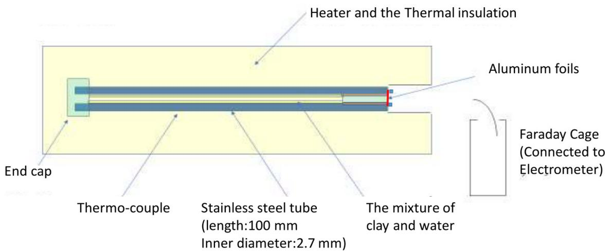
**Fig. 2.** Schematic diagram of experimental equipment to verify whether the mixture of clay and water is charged at high temperature and pressurized.
