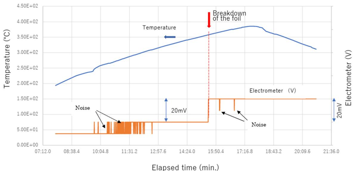
**Fig. 3.** Time-lapse change of the temperature and the Faraday cage (Electrometer) signal.
