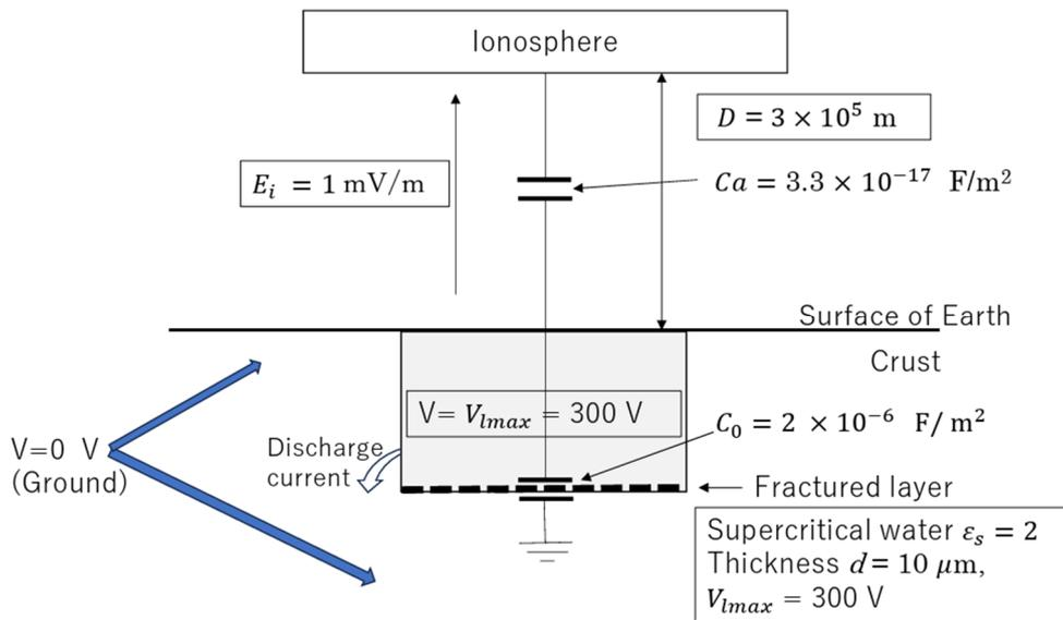
**Fig. 1.** The perturbation of the electric field  $E_i$  between the ionosphere and the fractured layer with supercritical water.  $E_i$  would superimpose to the original electric field for the global circuit. Numbers in the square are the assumed values for this capacitance coupling model.
