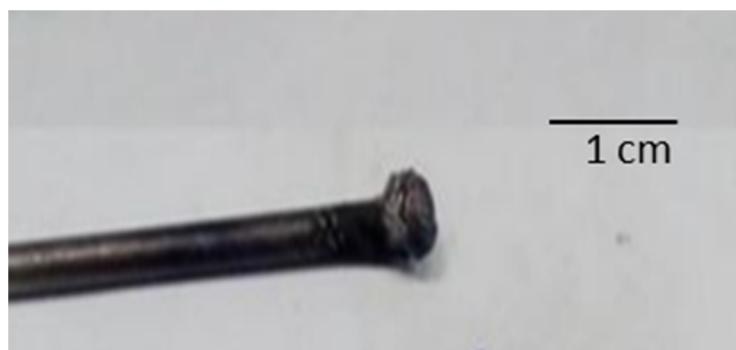
Fig. 3. Carbon black deposits on the tip of the rod electrode.
