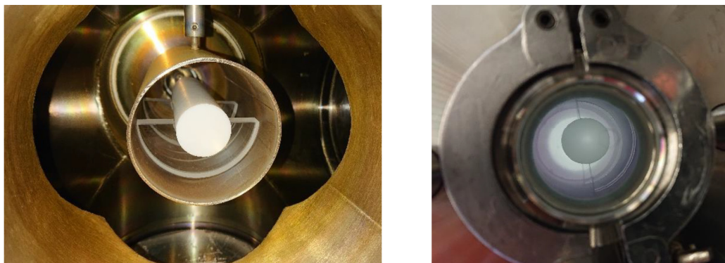
Fig. 3. On the left: opened plasma chamber with hollow cathode and PTFE-rod in its center. On the right: closed chamber, view from the outside through inspection window, oxygen plasma.
