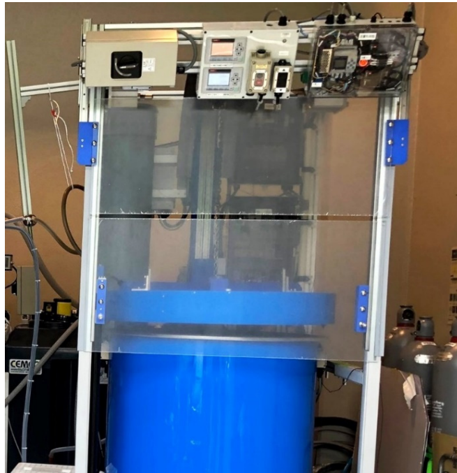
Fig. 7. Safety door at front of treatment tank.
