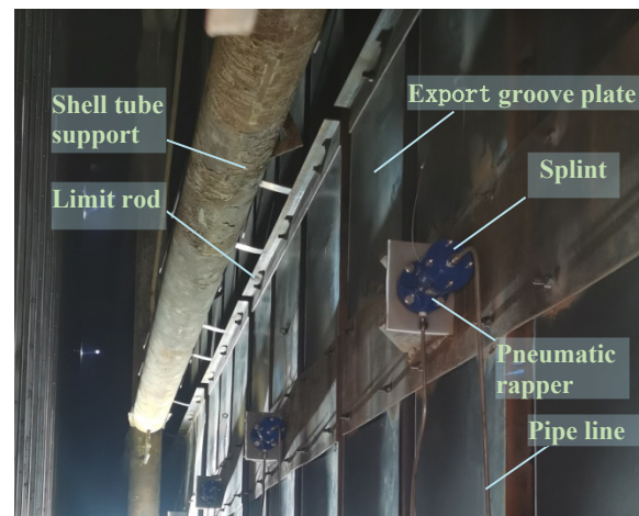
Fig.7. Small unit pneumatic vibration device
