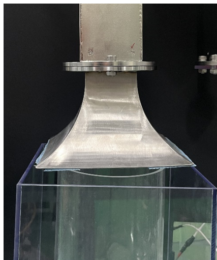
Fig. 6. Trumpet shaped duct installed at the bottom of the collection plate.
